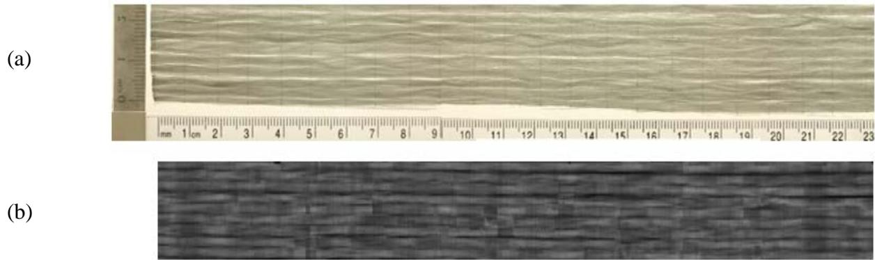
**Figure 1:** Image (a) is an original picture of the fibrous reinforcement. Image (b) shows the grey level mapping obtained after processing in order to evaluate the local fiber volume content.
