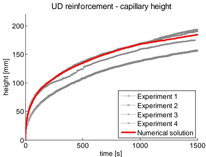
**Figure 1:** Capillary height as a function of time modelled with a saturation model
